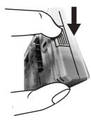
Push the groove of the thermostat housing
