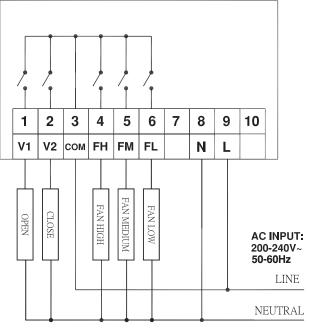
Contact Rating:  $\mu$  \_\_\_\_ 5(3)A/250~
