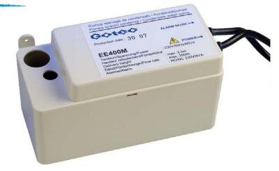
The centrifugal condensate pump EE400 is designed to automatically remove the liquid from an air-conditioner and evaporator coil. This pump is made from a tough ABS plastic body so it will withstand corrosion and impact. The internal pump unit can be used in an external pan as well (maximum pan height 70 mm).
