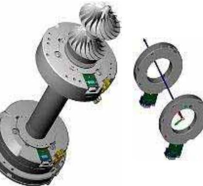
Two radial and one axial bearings are used.
